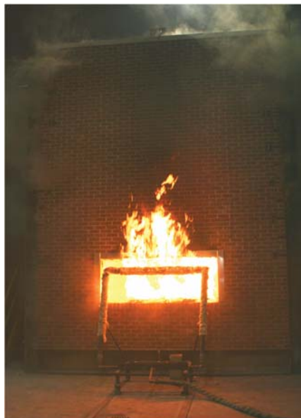
Fire emitting from the NFPA 285 test window.
