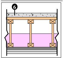
Adding 1 ½ inch layer of concrete or gypsum-concrete improves the airborne noise resistance, but it reduces the impact noise resistance. A bonded cementitious topping will enable a direct sound transmission path.
