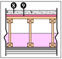
Research testing shows that using QuietZone<sup>TM</sup> Acoustic Floor Mat as a resilient interlayer and bond breaker clearly provides superior reductions in both airborne and structure-borne noise.
