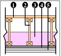
An untreated floor assembly provides only marginal acoustic resistance to airborne (FSTC) and structure-borne impact (FIIC) noise.
