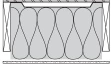
Standard Batts compressed into a  $114^{\prime\prime}$  cavity with ventilation baffle added to allow 1" air space deliver approximately R-35.
