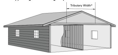
\*Tributary width is calculated as a percentage of the sum of the joist spans on either side of the wall: simple span: 0.5 ft x (left span + right span) continuous span: 0.625 ft x (left span + right span)
