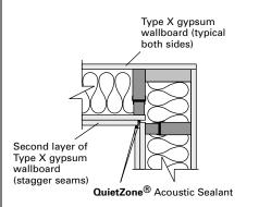
Apply **QuietZone**<sup>®</sup> Acoustic Sealant along corner of first layer of Type X gypsum wallboard before applying second layer of Type X gypsum wallboard.
